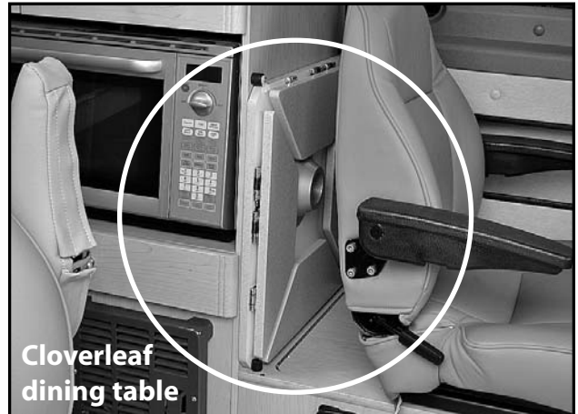
Picture B-P3: Lower galley cabinet showing location of cloverleaf table, (stored position).
