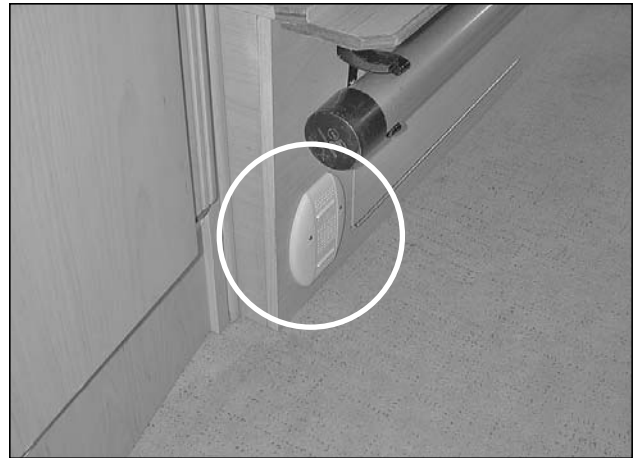
Picture F-P1: Propane leak detector.
