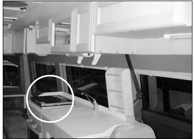
Picture B-P25: Lifting stove top cover.
