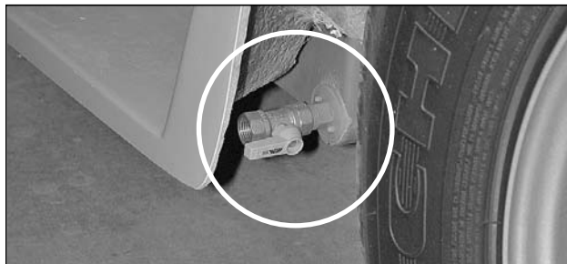
Picture B-P31: Location of the exterior fresh water tank drain valve (open position).
