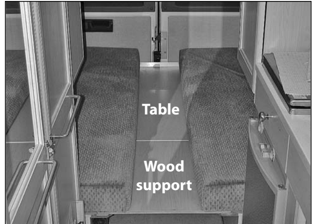
Picture B-P10: Placement of the table top and the wood support for the king size bed.
