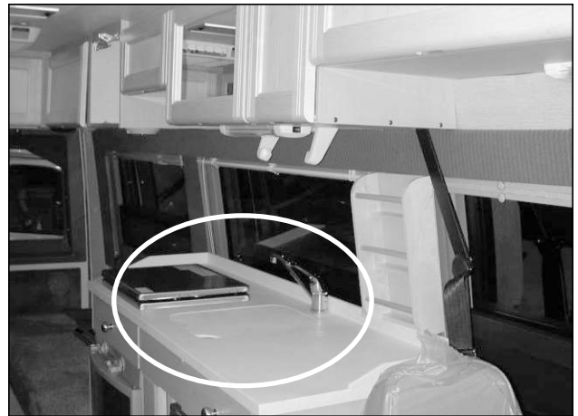
Picture B-P26: Counter top with sink cover in place.
